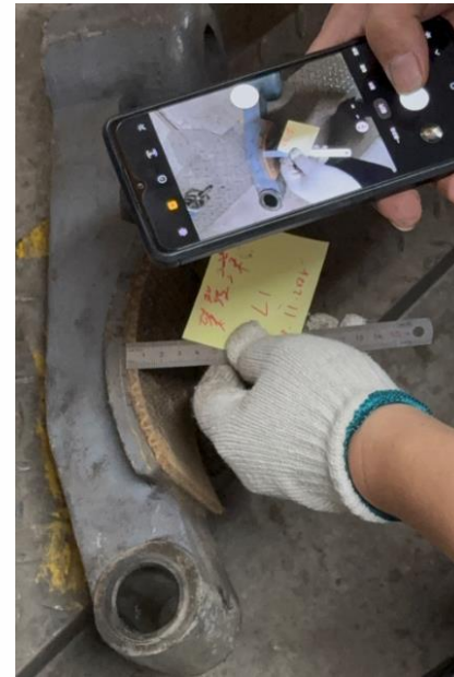
Measure the Lining
